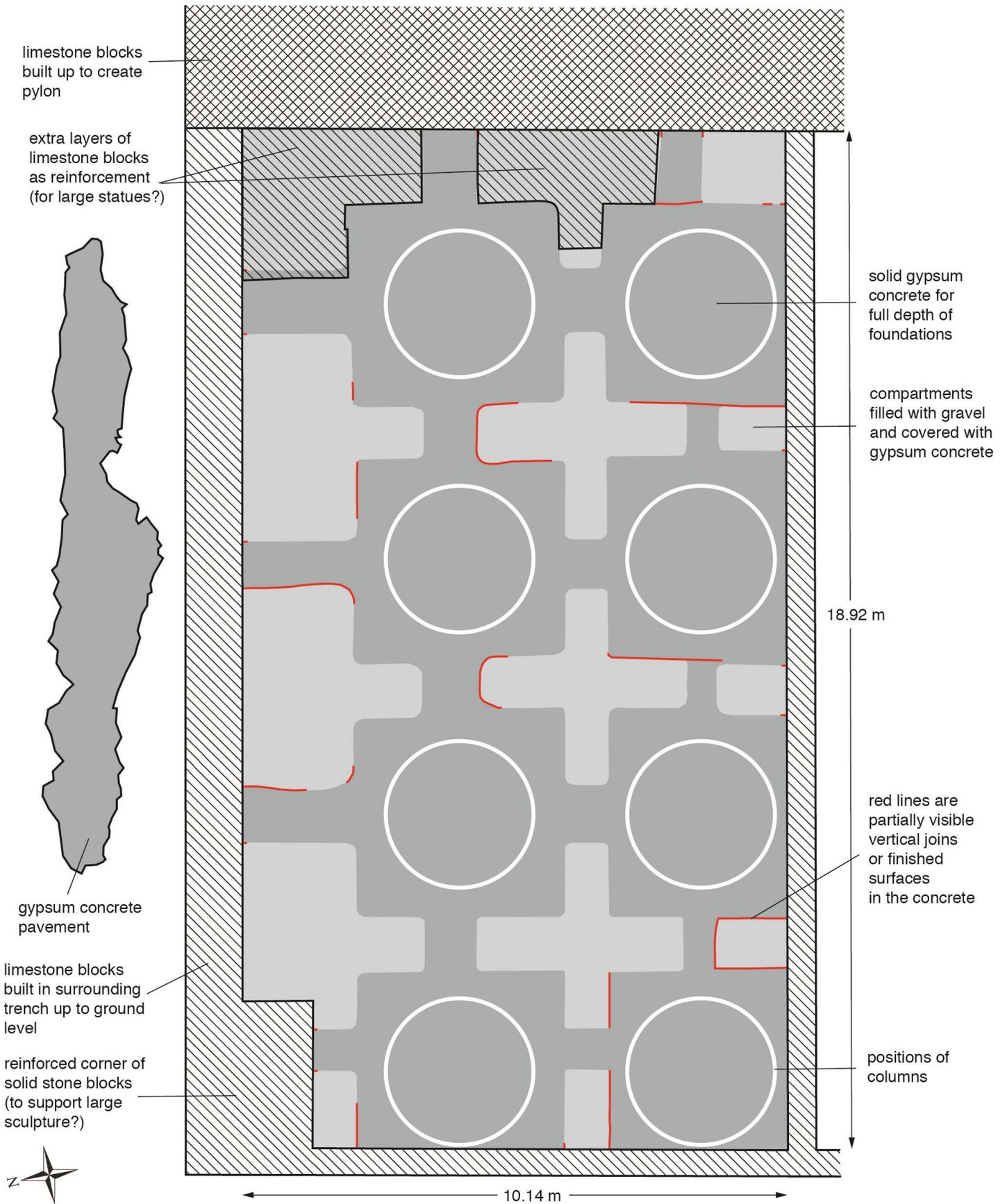
Figure 6. Outline plan of the north gypsum platform in front of the first stone pylon of the temple, showing the main constructional elements.
